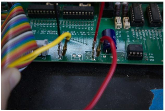
15. Connect the white end of the new power cable to the Z-Turn board:
