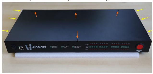
3. Remove all six of the side screws. The yellow arrows in the above picture mark these.
