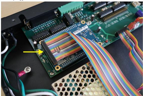
6. Put fingers under each of the four corners of the DE0-Nano, and gently wiggle it up out of the sockets.
