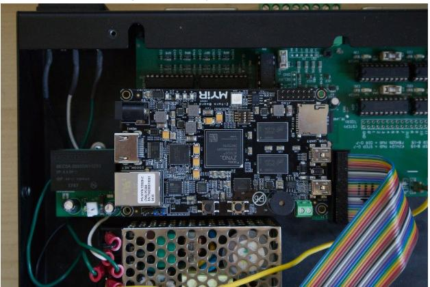
9. Attach the black end of the ribbon connector. Again, make sure the pins are lined up properly before you push it securely into place. It will be tight, but it should fit.
