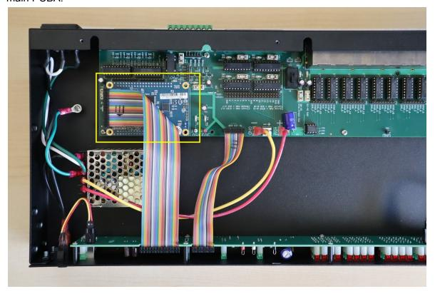
5. Carefully wiggle the black end of the rainbow connector to remove it from the DE0-Nano.
