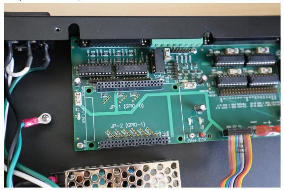
8. Insert the new Z-Turn very carefully into the slots. Refer to the picture below to make sure you have it oriented properly. Make sure all of the pins are lined up with the two bottom sockets before pushing it down securely.
